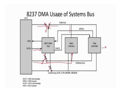
So, this is the scenario, you can see something like that; say this is the DMA controller, initially what will happen just you think that processor is directly connected to the main memory with this particular bus ok. This is the address bus, this is the, this is the data bus. So, processor is working with this particular memory.
