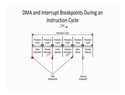
So, this is the DMA and interrupt breakpoints you can say. So, what is the interrupt breakpoint, basically when these breakpoint, basically what we are saying that when the processor is going to suspend its current program execution. So, if interrupt is coming. Say, currently it is executing one particular instruction then what will happen? It is going to complete this instruction and at that time after completion of the instruction it will check whether any
