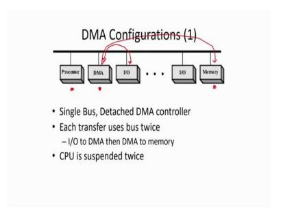
Now how you are going to connect those particular DMA controller. So, these are simple. So, this is a single bus, we detached DMA controller. So, in the particular user, see this is the processor. Processor is directly connected to the memory through this particular system bus. So, now processor can transfer information from memory.
